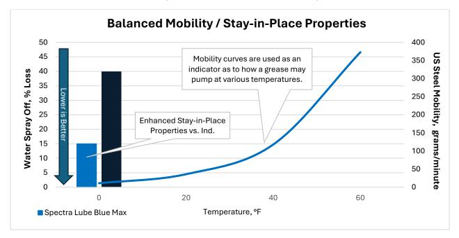
The left side of the chart is the Water Spray Off test results, which is a good indicator of the adhesive properties. Spectra Lube Blue Max polymer architecture provides excellent "stay-in-place" properties while carefully balancing its ability to pump in a broad range of temperatures.
