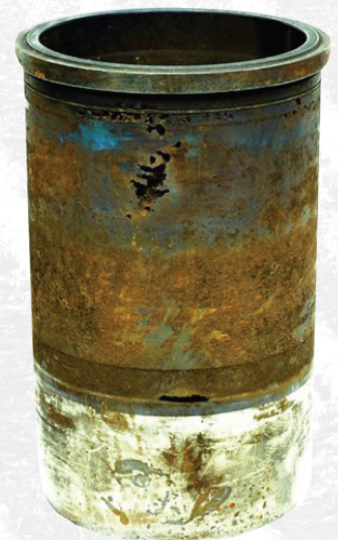
Cylinder with liner cavitation
